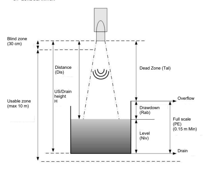
The level of liquid to be measured must be within the usable zone.
