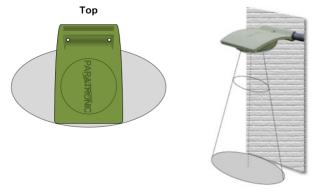
The CR420 radar sensor is fixed directly onto a horizontal tube of outside diameter  $\leq 40$  mm (or by using the optional "Radar bracket"). It is held in position by an 8 mm diameter screw.
